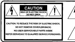
This symbol warns the user that uninsulated voltage within the unit may have sufficient magnitude to cause electric shock. Therefore, it is dangerous to make any kind of contact with any inside part of this unit.
